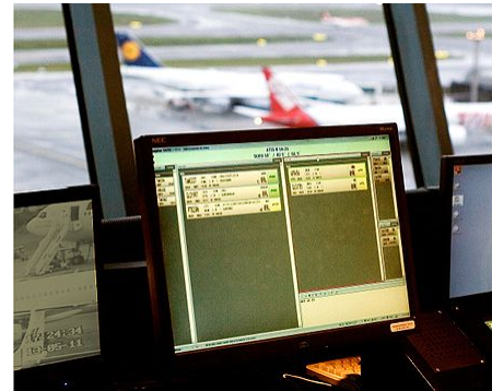
Electronic flight progress strip system at São Paulo Intl. control tower – ground control
